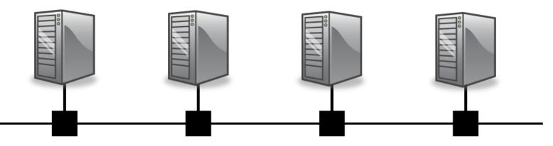
All hosts transmit & receive on one channel Packets are of variable size.
