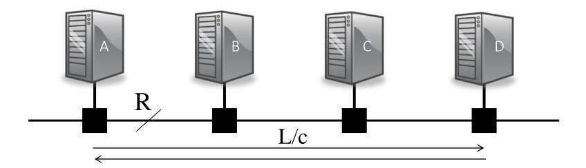
For an end host to detect a collision before it finishes transmitting a packet, we require:
